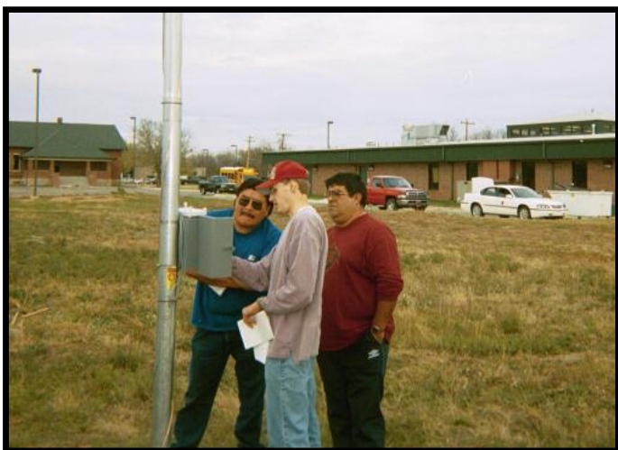
Moran Bibles (left) and John Norman (right) of the Otoe-Missouria Tribe work with Troy Simonsen to set up the datalogger on the 20-meter tower.
